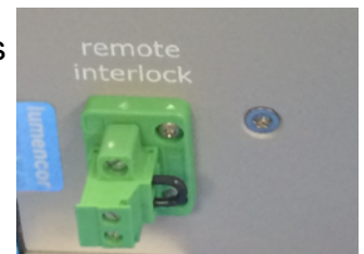
Figure 5. Remote interlock jumper inserted in the labeled receptacle on the lower left side of the rear panel of the light engine.
