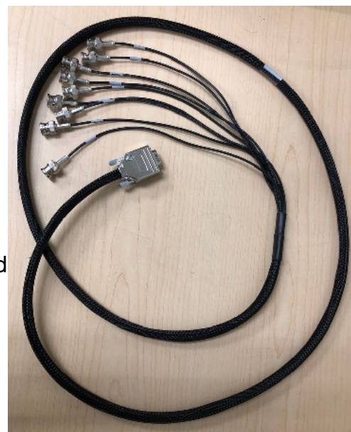
Figure 6. BNC breakout cable to enable TTL triggering
