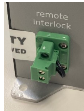
Figure 5. Remote interlock jumper inserted in the labeled receptacle on the lower left side of the rear panel of the light engine.
