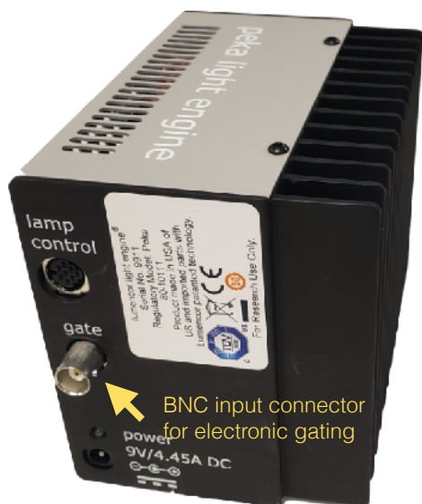
Figure 3. Rear panel of PEKA light engine configured for remote control from Nikon microscope base.
