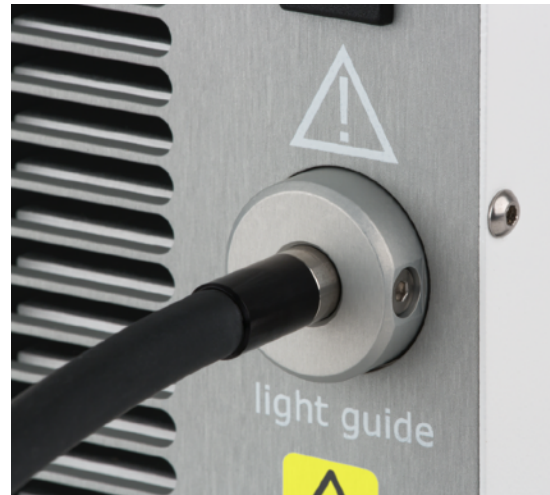
Figure 2. 3 mm diameter liquid light guide inserted in front panel light output port.
