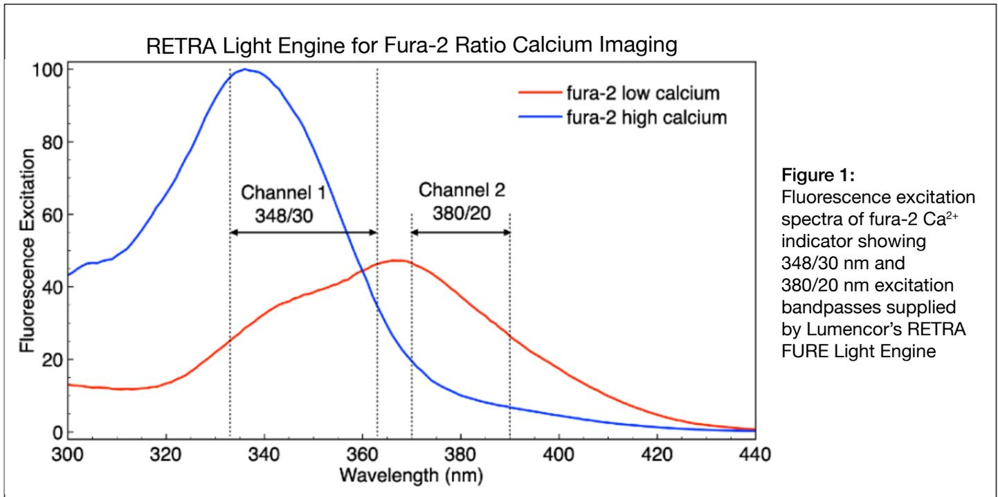
**Figure 1:** Fluorescence excitation spectra of fura-2 Ca<sup>2+</sup> indicator showing 348/30 nm and 380/20 nm excitation bandpasses supplied by Lumencor’s RETRA FURE Light Engine
