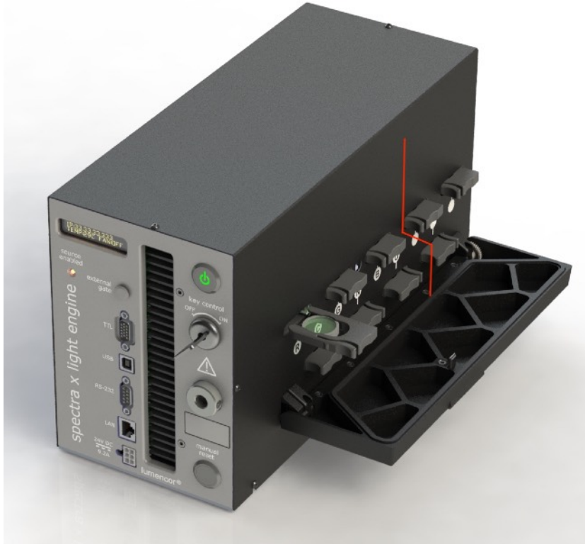
Figure 9. SPECTRA X filter compartment with hinged access cover open and the red (635/22 nm) filter extracted. The red line marks the boundary between the six operational filter slots and the 3 rearmost slots used for non-operational storage.
