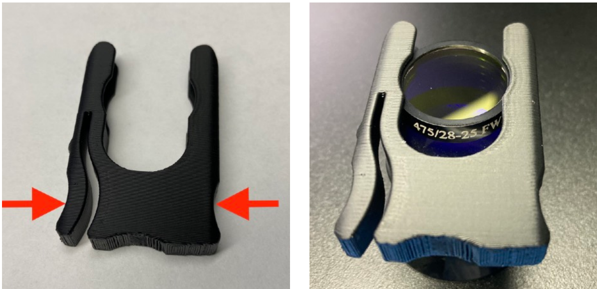
Figure 10. SPECTRA X filter holders. Left: Empty holder. Squeeze at the points indicated by the red arrows while pulling outwards to release the filter holder from the light engine. Right: Holder showing correct insertion of a filter and the bandpass specification (475/28 nm) marked on the filter.
