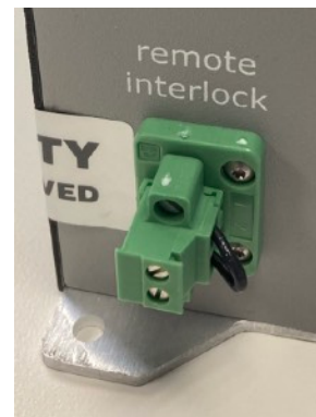
Figure 4. Remote interlock jumper inserted in the labeled receptacle on the lower left side of the rear panel of the light engine.
