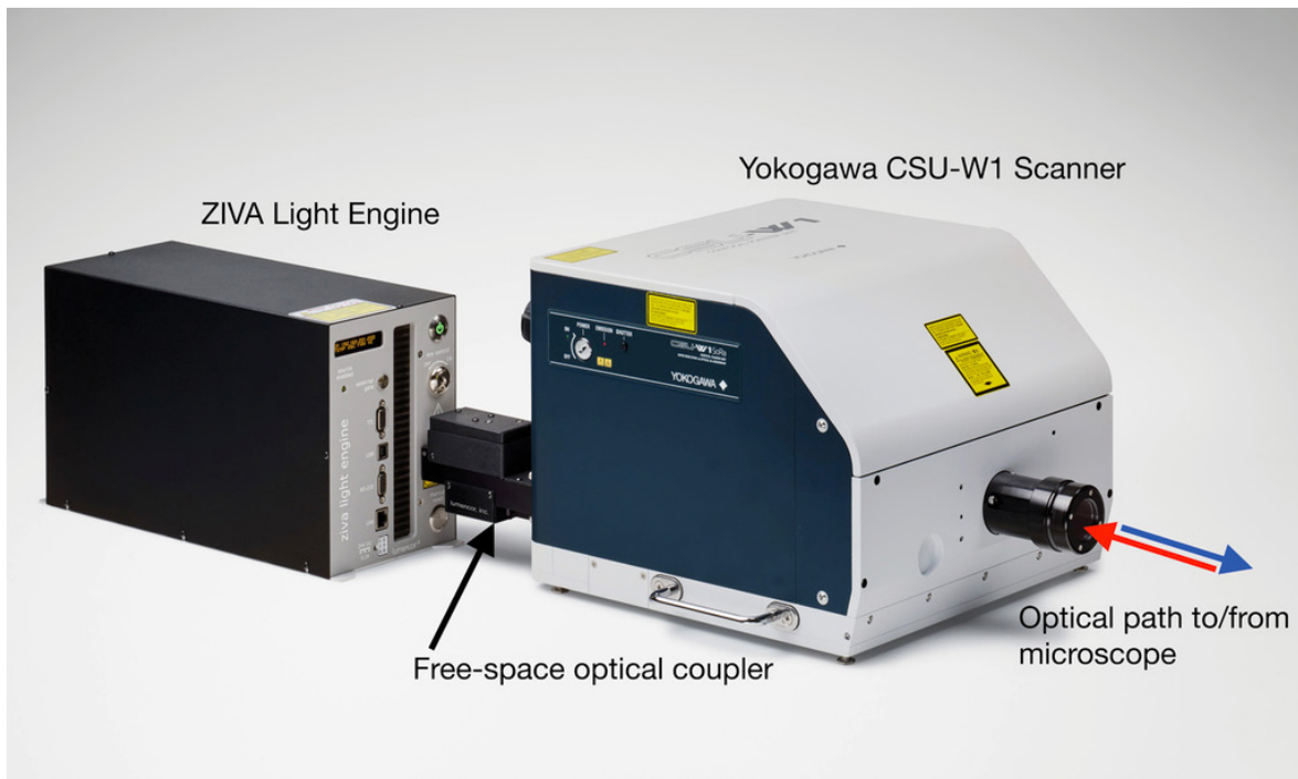
Figure 2. Layout of the ZIVA Light Engine coupled to the Yokogawa CSU confocal scanner.
