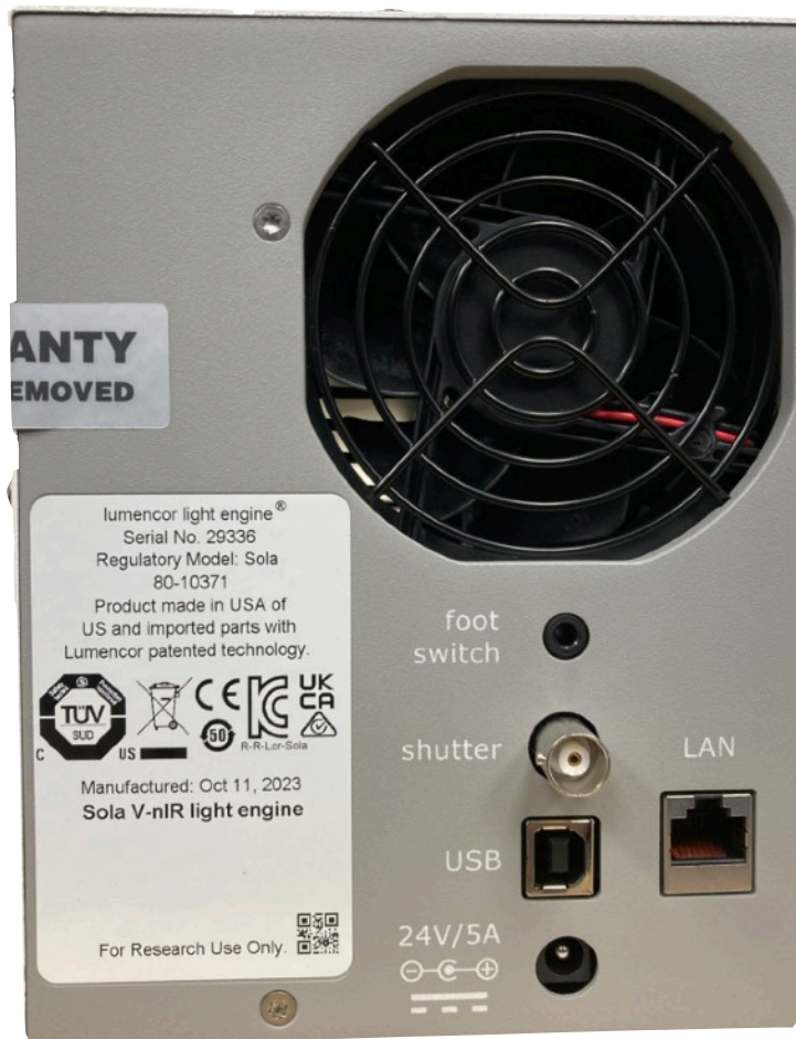
Figure 1. SOLA Light Engine rear panel. The serial number of the light engine shown is 29336 . The rear panel also carries the input connections for the optional foot switch controller, the electronic shutter , USB control devices and ethernet access to the onboard control GUI ( LAN , only on units manufactured after August 2023). The input connection for the DC power supply is labeled 24V/5A . The air cooling exhaust port is located at the upper right.
