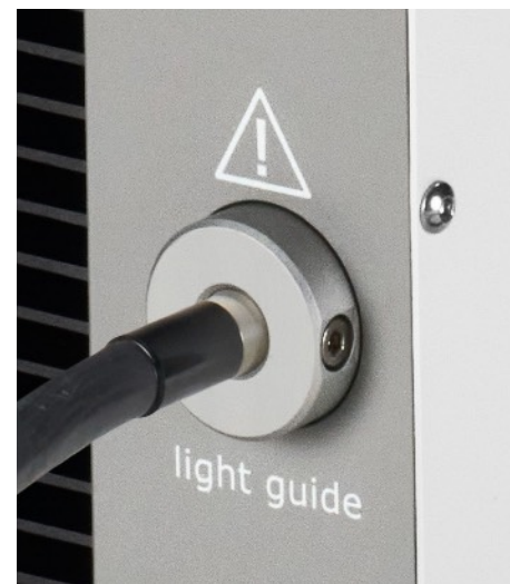
Figure 3. 3 mm diameter liquid light guide inserted in front panel light output port.
